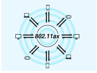
TWT (Target Wake-up Time). 802.11ax support TWT, allowing devices to negotiate when need to wake up, send and receive data. In additional, wireless AP can group the device into different TWT cycles, increase sleep time, reduce the device competing after wake-up, and save the device power.
